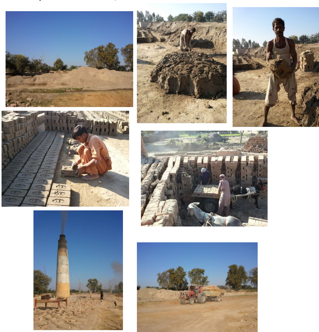
Figure 1: Brick making process left to right then below: Clay preparation for brick; pera making for bricks; mud brick preparation by taking out of the mould; sun drying the mud bricks; Transportation to kiln; Baking mud bricks in the kiln; transportation to market.
